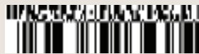
GS1 DataBar Composite is one of a few symbologies that combine 1D and 2D elements in a single bar code symbol.
